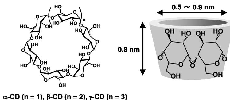
**Figure 1.** Structures of cyclodextrins (CDs).
