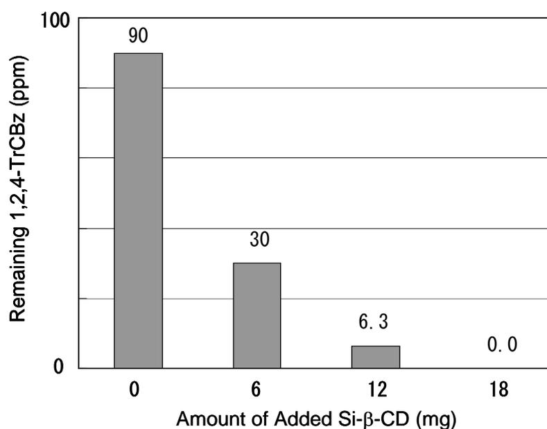
**Figure 4.** Relationship between the amount of 1,2,4-TrCBz remaining in insulating oil (242 mg) and the amount of added Si-β-CD. Initial concentration of 1,2,4-TrCBz was 90 ppm.
